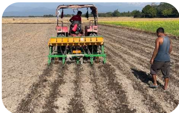
Sowing of maize crop with zero tillage machine under non-residue and residue management practices.
