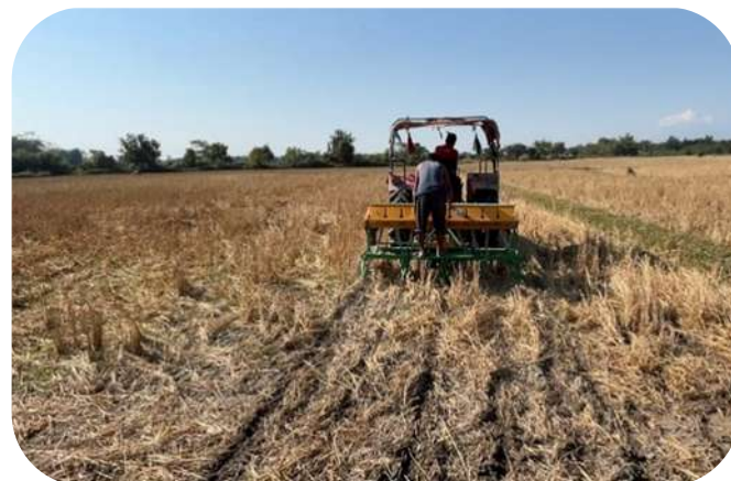
Sowing of maize crop with zero tillage machine under non-residue and residue management practices.
